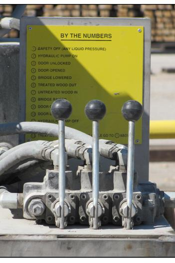
Remote control assembly for locking ring, swing cylinder, and bridge rails.
