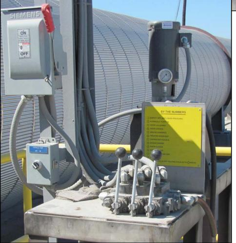
Remote control assembly for locking ring, swing cylinder, and bridge rails.
